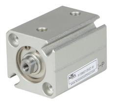
NITRA pneumatic cylinder, compact extruded, 16mm bore, 8mm rod diameter, 10mm stroke, double acting, magnetic piston, tapped end caps mount.
