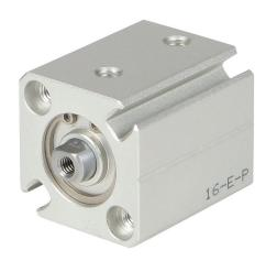
NITRA pneumatic cylinder, compact extruded, 16mm bore, 8mm rod diameter, 5mm stroke, double acting, magnetic piston, tapped end caps mount.
