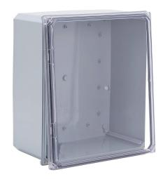
Integra Premium series enclosure, NEMA 1/2/3/3R/3S/4/4X/5/6/6P/12/13,  $16 \times 14 \times 7$  in (HxWxD), wall mount, polycarbonate, gray, gloss finish, clear polycarbonate screw cover.
