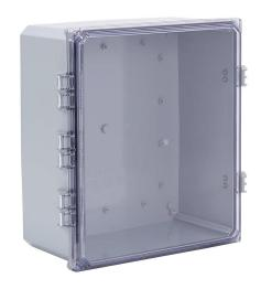
Integra Premium series enclosure, NEMA 1/2/3/3R/3S/4/4X/5/12/13, 16 x 14 x 7in (HxWxD), wall mount, polycarbonate, gray, gloss finish, clear polycarbonate single-door, glass-filled nylon quick-release latch, padlock hasp and staple.
