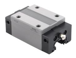
WON H15 series standard bearing block, full ball recirculating bearing, rectangular, end seal and inside seal, carbon steel. For use with H15 series rails.
