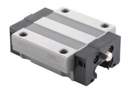
WON H15 series standard bearing block, full ball recirculating bearing, flanged, end seal, carbon steel. For use with H15 series rails.
