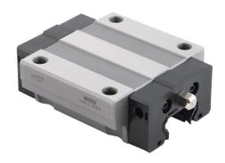
WON H15 series standard bearing block, full ball recirculating bearing, flanged, end seal and inside seal, carbon steel. For use with H15 series rails.
