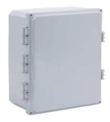
Integra Premium series enclosure, NEMA 1/2/3/3R/3S/4/4X/5/12/13, 14 x 12 x 6in (HxWxD), wall mount, polycarbonate, gray, gloss finish, single-door, glass-filled nylon quick-release latch, padlock hasp and staple.
