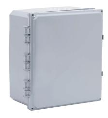
Integra Premium series enclosure, NEMA 1/2/3/3R/3S/4/4X/5/6/6P/12/13, 14 x 12 x 6in (HxWxD), wall mount, polycarbonate, gray, gloss finish, hinged screw cover.
