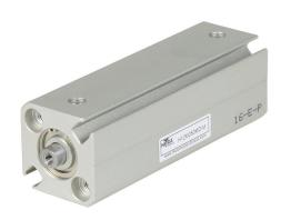
NITRA pneumatic cylinder, compact extruded, 12mm bore, 6mm rod diameter, 50mm stroke, double acting, magnetic piston, tapped end caps mount.
