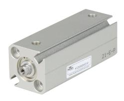
NITRA pneumatic cylinder, compact extruded, 12mm bore, 6mm rod diameter, 40mm stroke, double acting, magnetic piston, tapped end caps mount.
