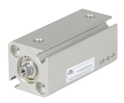
NITRA pneumatic cylinder, compact extruded, 12mm bore, 6mm rod diameter, 30mm stroke, double acting, magnetic piston, tapped end caps mount.
