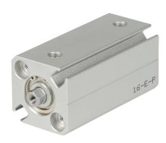
NITRA pneumatic cylinder, compact extruded, 12mm bore, 6mm rod diameter, 25mm stroke, double acting, magnetic piston, tapped end caps mount.
