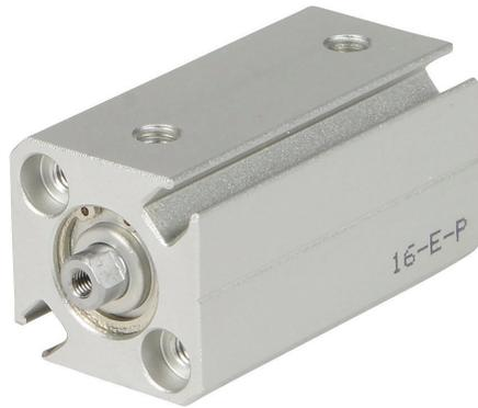
NITRA pneumatic cylinder, compact extruded, 12mm bore, 6mm rod diameter, 20mm stroke, double acting, magnetic piston, tapped end caps mount.
