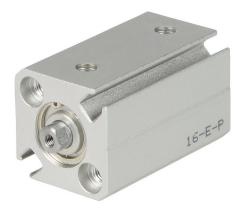
NITRA pneumatic cylinder, compact extruded, 12mm bore, 6mm rod diameter, 15mm stroke, double acting, magnetic piston, tapped end caps mount.
