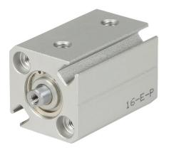
NITRA pneumatic cylinder, compact extruded, 12mm bore, 6mm rod diameter, 10mm stroke, double acting, magnetic piston, tapped end caps mount.
