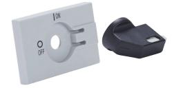
Merz rotary handle, pistol, black/gray, direct mount, 2-position, lockable in OFF only, NEMA 1. For use with Merz ML3 switch bodies in DIN rail applications. On-off faceplate included.
