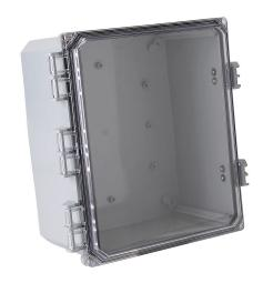
Integra Premium series enclosure, NEMA 1/2/3/3R/3S/4/4X/12/13, 12 x 10 x 6in (HxWxD), wall mount, polycarbonate, light gray, gloss finish, clear polycarbonate singledoor, glass-filled nylon quick-release latch, padlock hasp and staple.
