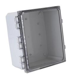
Integra Premium series enclosure, NEMA 1/2/3/3R/3S/4/4X/6/6P/12/13,  $12 \times 10 \times 6$ in (HxWxD), wall mount, polycarbonate, light gray, gloss finish, clear polycarbonate hinged screw cover.
