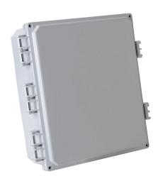
Integra Premium series enclosure, NEMA 1/2/3/3R/3S/4/4X/12/13, 12 x 10 x 4in (HxWxD), wall mount, polycarbonate, light gray, gloss finish, single-door, glass-filled nylon quick-release latch, padlock hasp and staple.
