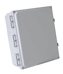
Integra Premium series enclosure, NEMA 1/2/3/3R/3S/4/4X/6/6P/12/13, 12 x 10 x 4in (HxWxD), wall mount, polycarbonate, light gray, gloss finish, hinged screw cover.
