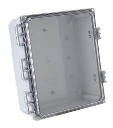
Integra Premium series enclosure, NEMA 1/2/3/3R/3S/4/4X/12/13, 12 x 10 x 4in (HxWxD), wall mount, polycarbonate, light gray, gloss finish, clear polycarbonate singledoor, glass-filled nylon quick-release latch, padlock hasp and staple.
