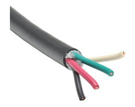
Helukabel portable cord, unshielded, SOOW, 600V, 4 conductors (includes ground), 18 AWG, EPDM thermoset rubber conductor insulation material, black, white, red and green, CPE thermoset rubber jacket, black, cut to length.
