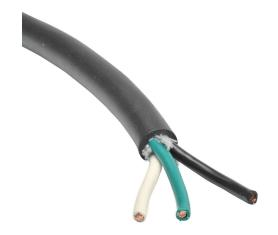
Helukabel portable cord, unshielded, SOOW, 600V, 3 conductors (includes ground), 18 AWG, EPDM thermoset rubber conductor insulation material, black, white and green, CPE thermoset rubber jacket, black, cut to length.
