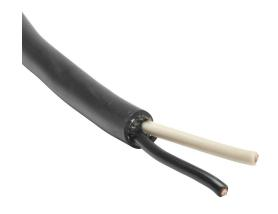
Helukabel portable cord, unshielded, SOOW, 600V, 2 conductors, 18 AWG, EPDM thermoset rubber conductor insulation material, black and white, CPE thermoset rubber jacket, black, cut to length.
