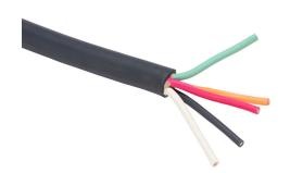
Helukabel portable cord, unshielded, SOOW, 600V, 5 conductors (includes ground), 16 AWG, EPDM thermoset rubber conductor insulation material, black, white, red, green and orange, CPE thermoset rubber jacket, black, cut to length.
