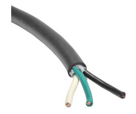
Helukabel portable cord, unshielded, SOOW, 600V, 3 conductors (includes ground), 16 AWG, EPDM thermoset rubber conductor insulation material, black, white and green, CPE thermoset rubber jacket, black, cut to length.
