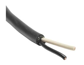
Helukabel portable cord, unshielded, SOOW, 600V, 2 conductors, 16 AWG, EPDM thermoset rubber conductor insulation material, black and white, CPE thermoset rubber jacket, black, cut to length.
