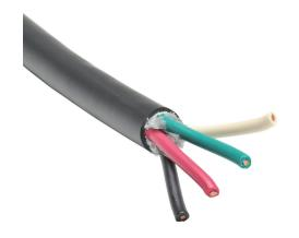
Helukabel portable cord, unshielded, SOOW, 600V, 4 conductors (includes ground), 14 AWG, EPDM thermoset rubber conductor insulation material, black, white, red and green, CPE thermoset rubber jacket, black, cut to length.
