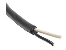
Helukabel portable cord, unshielded, SOOW, 600V, 2 conductors, 14 AWG, EPDM thermoset rubber conductor insulation material, black and white, CPE thermoset rubber jacket, black, cut to length.
