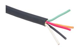
Helukabel portable cord, unshielded, SOOW, 600V, 5 conductors (includes ground), 12 AWG, EPDM thermoset rubber conductor insulation material, black, white, red, green and orange, CPE thermoset rubber jacket, black, cut to length.
