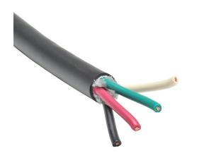
Helukabel portable cord, unshielded, SOOW, 600V, 4 conductors (includes ground), 12 AWG, EPDM thermoset rubber conductor insulation material, black, white, red and green, CPE thermoset rubber jacket, black, cut to length.
