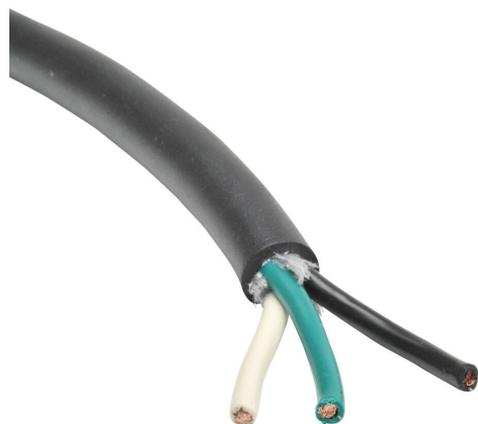
Helukabel portable cord, unshielded, SOOW, 600V, 3 conductors (includes ground), 12 AWG, EPDM thermoset rubber conductor insulation material, black, white and green, CPE thermoset rubber jacket, black, cut to length.
