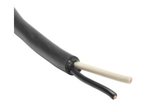
Helukabel portable cord, unshielded, SOOW, 600V, 2 conductors, 12 AWG, EPDM thermoset rubber conductor insulation material, black and white, CPE thermoset rubber jacket, black, cut to length.
