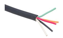
Helukabel portable cord, unshielded, SOOW, 600V, 5 conductors (includes ground), 10 AWG, EPDM thermoset rubber conductor insulation material, black, white, red, green and orange, CPE thermoset rubber jacket, black, cut to length.
