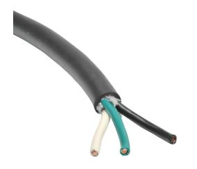
Helukabel portable cord, unshielded, SJOOW, 300V, 3 conductors (includes ground), 18 AWG, EPDM thermoset rubber conductor insulation material, black, white and green, CPE thermoset rubber jacket, black, cut to length.
