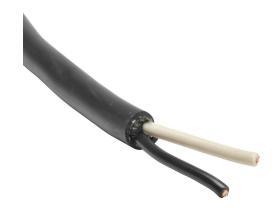
Helukabel portable cord, unshielded, SJOOW, 300V, 2 conductors, 18 AWG, EPDM thermoset rubber conductor insulation material, black and white, CPE thermoset rubber jacket, black, cut to length.
