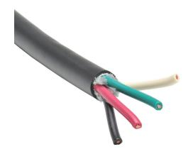
Helukabel portable cord, unshielded, SJOOW, 300V, 4 conductors (includes ground), 16 AWG, EPDM thermoset rubber conductor insulation material, black, white, red and green, CPE thermoset rubber jacket, black, cut to length.
