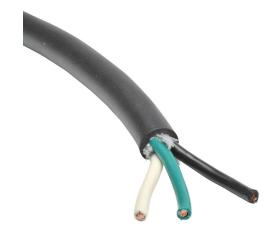
Helukabel portable cord, unshielded, SJOOW, 300V, 3 conductors (includes ground), 16 AWG, EPDM thermoset rubber conductor insulation material, black, white and green, CPE thermoset rubber jacket, black, cut to length.
