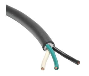
Helukabel portable cord, unshielded, SJOOW, 300V, 3 conductors (includes ground), 14 AWG, EPDM thermoset rubber conductor insulation material, black, white and green, CPE thermoset rubber jacket, black, cut to length.
