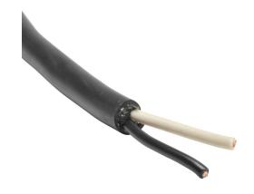
Helukabel portable cord, unshielded, SJOOW, 300V, 2 conductors, 14 AWG, EPDM thermoset rubber conductor insulation material, black and white, CPE thermoset rubber jacket, black, cut to length.
