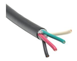
Helukabel portable cord, unshielded, SJOOW, 300V, 4 conductors (includes ground), 12 AWG, EPDM thermoset rubber conductor insulation material, black, white, red and green, CPE thermoset rubber jacket, black, cut to length.
