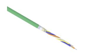
Helukabel HELUKAT continuous flexing Profinet Type R cable, overall shielded, 1 star quad, 22 AWG, 19-stranded, tinned copper, polyolefin conductor insulation material, PUR jacket, green, cut to length.
