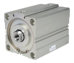
NITRA pneumatic cylinder, compact extruded, 100mm bore, 32mm rod diameter, 100mm stroke, double acting, magnetic piston, tapped end caps mount.
