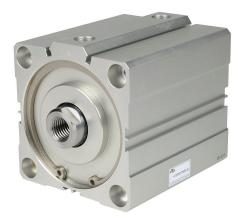
NITRA pneumatic cylinder, compact extruded, 100mm bore, 32mm rod diameter, 75mm stroke, double acting, magnetic piston, tapped end caps mount.
