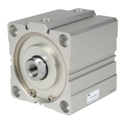
NITRA pneumatic cylinder, compact extruded, 100mm bore, 32mm rod diameter, 50mm stroke, double acting, magnetic piston, tapped end caps mount.
