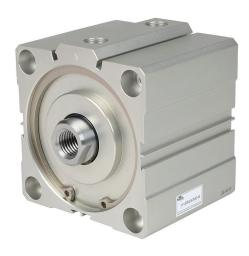
NITRA pneumatic cylinder, compact extruded, 100mm bore, 32mm rod diameter, 40mm stroke, double acting, magnetic piston, tapped end caps mount.
