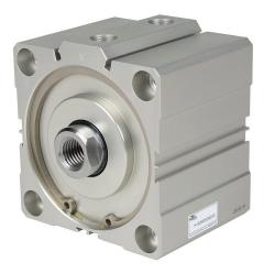
NITRA pneumatic cylinder, compact extruded, 100mm bore, 32mm rod diameter, 30mm stroke, double acting, magnetic piston, tapped end caps mount.
