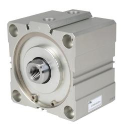
NITRA pneumatic cylinder, compact extruded, 100mm bore, 32mm rod diameter, 25mm stroke, double acting, magnetic piston, tapped end caps mount.
