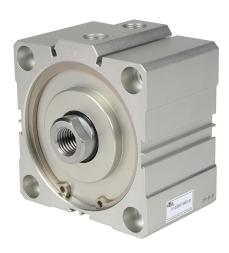
NITRA pneumatic cylinder, compact extruded, 100mm bore, 32mm rod diameter, 15mm stroke, double acting, magnetic piston, tapped end caps mount.
